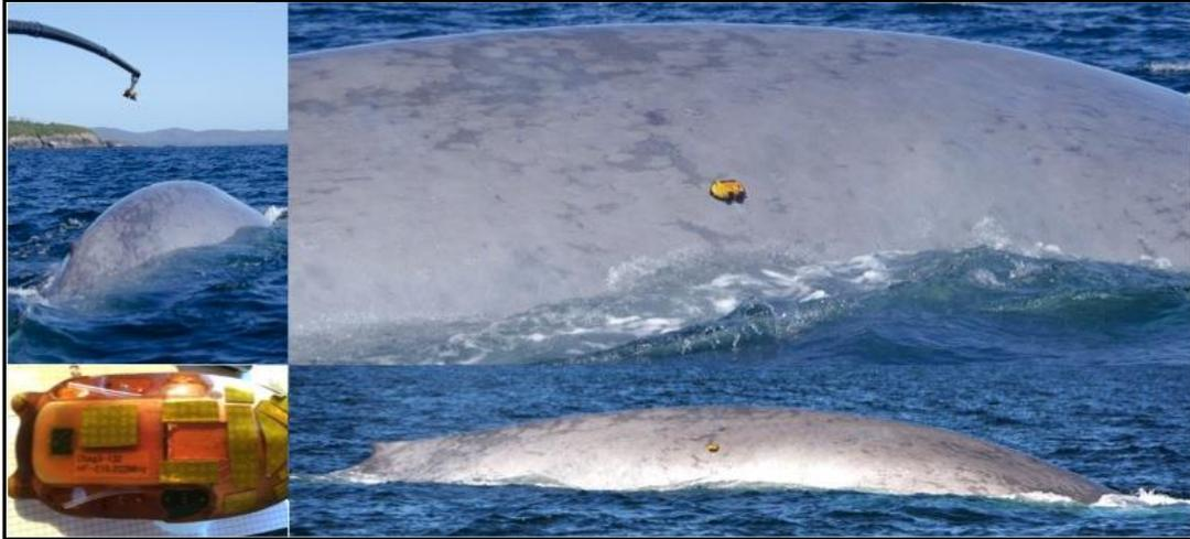
Figure 2. The DTAG (bottom left) and the attachment method via hand-held pole (top left); images on the right show the tag attached to a blue whale with its four suction cups and the tag's small size relative to the animal's size.
