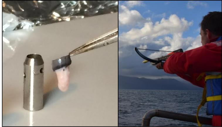
Figure 4. Stainless steel biopsy tips were used to collect skin and blubber samples. Biopsy bolts were deployed using a crossbow.
