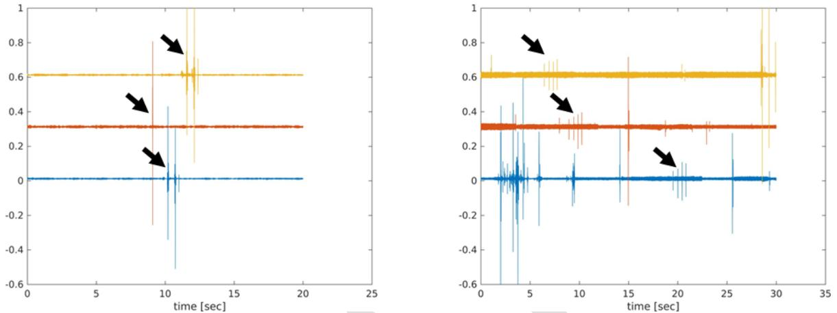
Figure 19. Time synchronization using clapping before (left) and after (right) of deployment. Arrows indicate claps; precise timing will be obtained by signal cross correlation and subsequent sample dropping.
