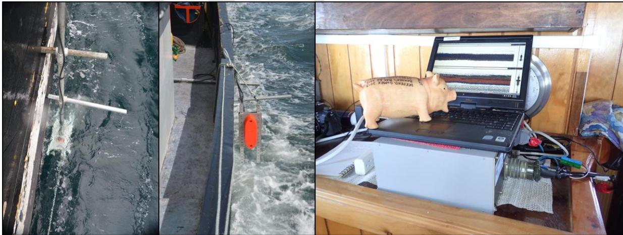
Figure 5. The scientific echosounder system was pole mounted on the port side of the RV Khronos for underway data collection (left) and could be raised for rapid transit (middle, the orange object is the transducer). The data collection and storage system were located on the bridge of the vessel (right, the pig is a lab mascot).
