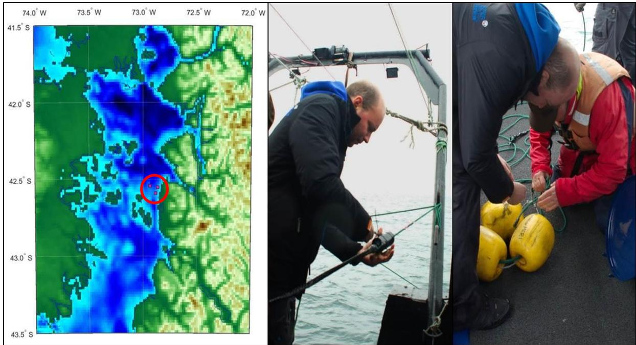
Figure 7. Location map of the PAM array in the Gulf of Ancud and preparation of a SoundTrap shallow water mooring.
